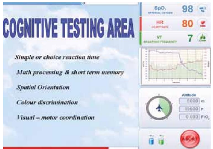
Fig. 2 Closeup of touch screen displaying physiological parameters oxygen saturation (SpO 2 ), Heart rate (HR) and ventilation frequency (Vt) in the top right quadrant, altitude and fractional inspired oxygen concentration (FIO 2 ) in the lower right quadrant and cognitive tests continuously displayed in the left half-screen. Note the ABORT button.
